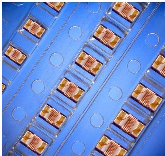
These high frequency High-Q chip inductors feature a monolithic body made of low loss ceramic wound with wire to achieve optimal high frequency performance.
