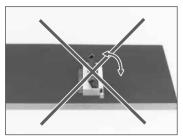
3) Application of excessive force to the inserted FPC/FFC may cause damage to connector and may affect the reliability of electrical connection.
