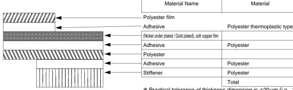
\* Practical tolerance of thickness dimension is  $\pm 20 \mu m$  (i.e., 187 to 227 $\mu m$ ).
