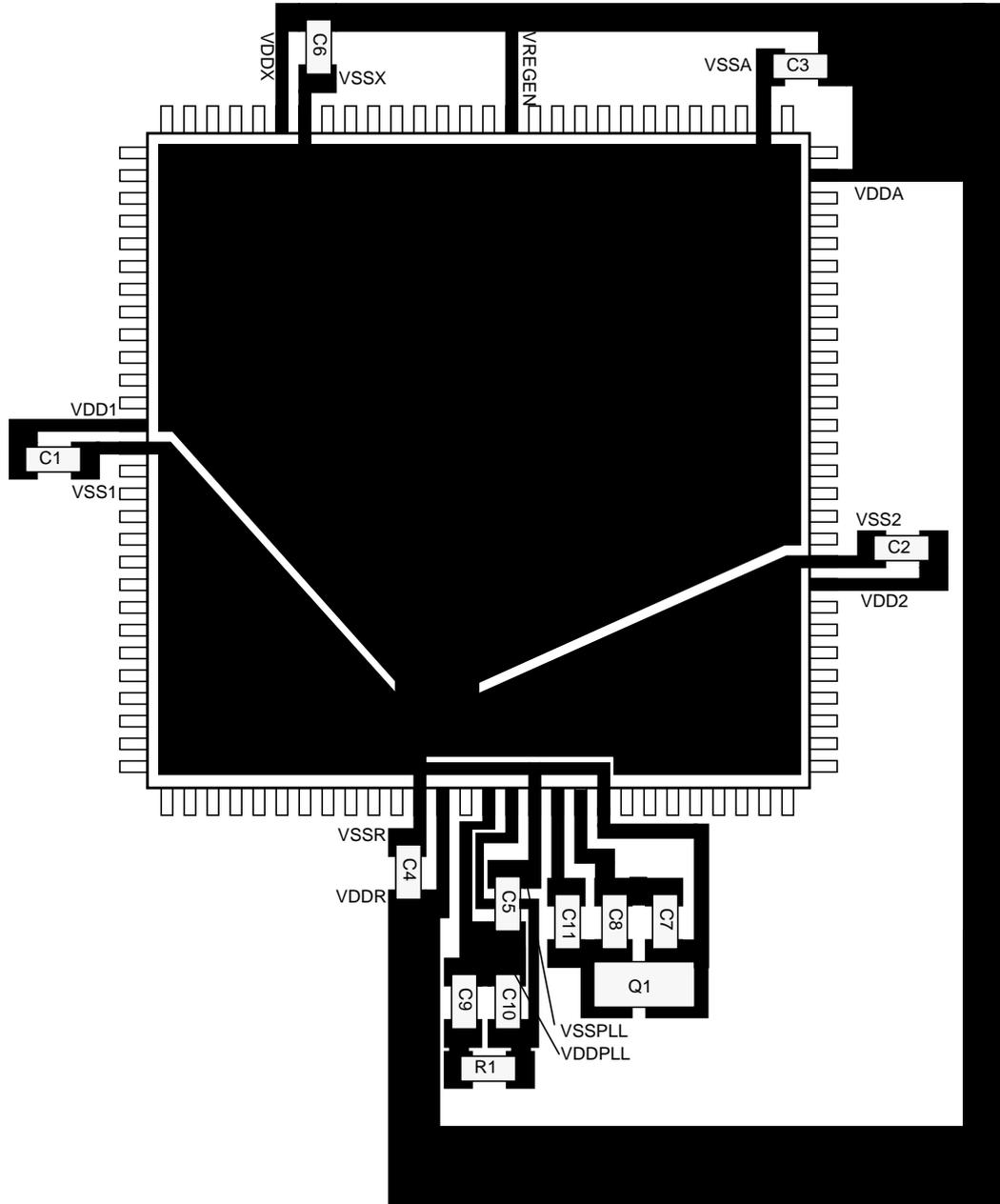
Figure 20-2 Recommended PCB Layout for 80QFP
