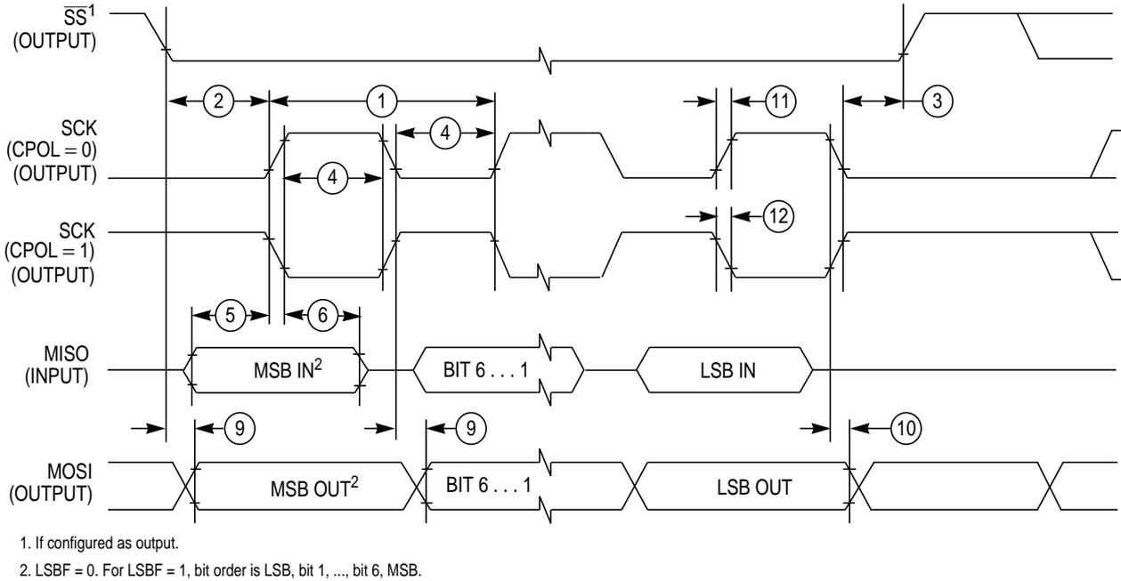
Figure A-5 SPI Master Timing (CPHA = 0)
