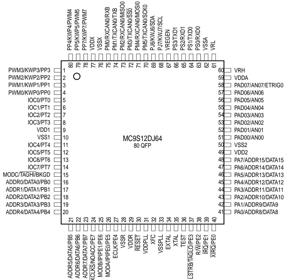
Figure 2-2 Pin Assignments in 80-pin QFP for MC9S12DJ64
