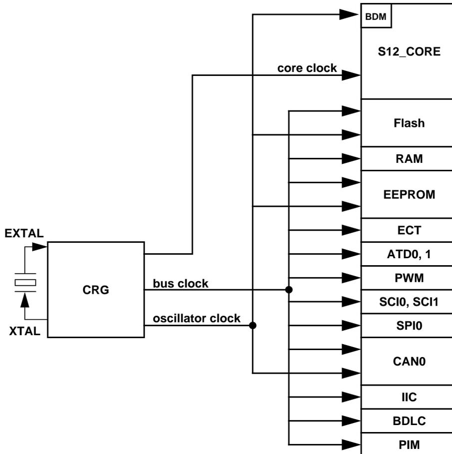
Figure 3-1 Clock Connections
