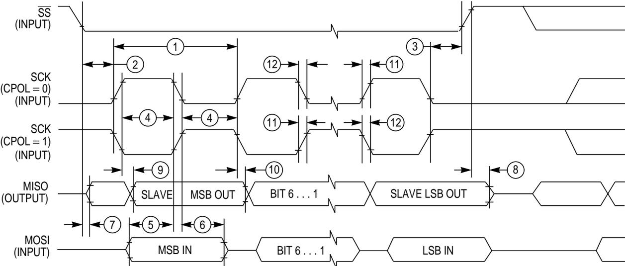
Figure A-8 SPI Slave Timing (CPHA = 1)
