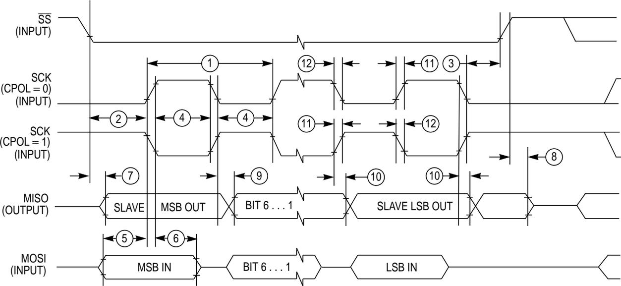
Figure A-7 SPI Slave Timing (CPHA = 0)
