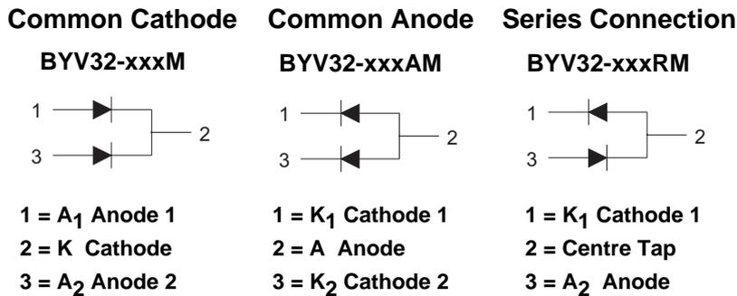
Applications include secondary rectification in high frequency switching power supplies.
