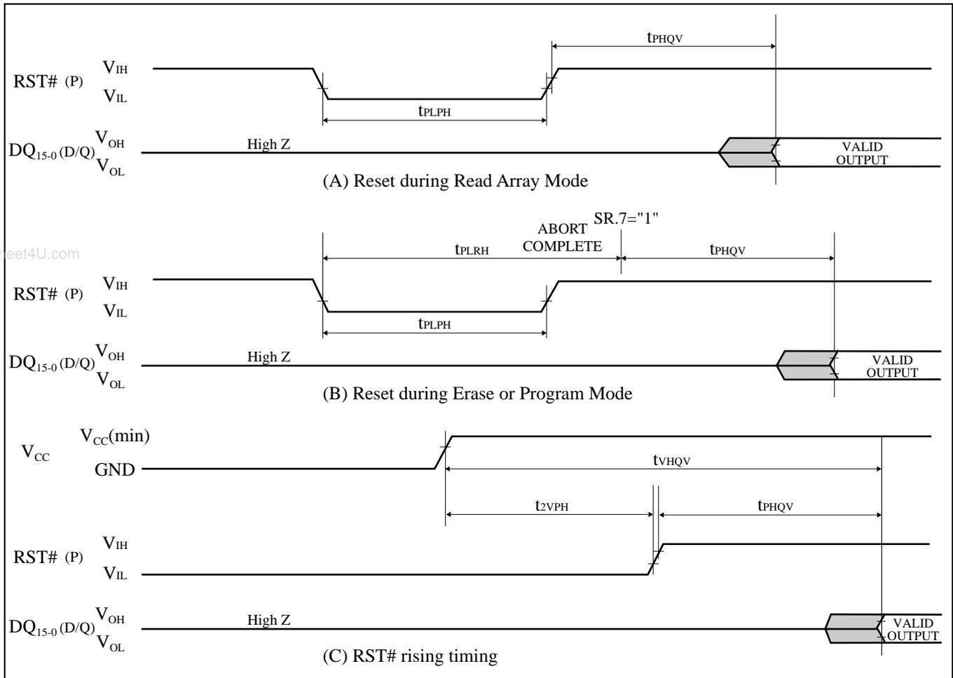
Figure 10. AC Waveform for Reset Operations
