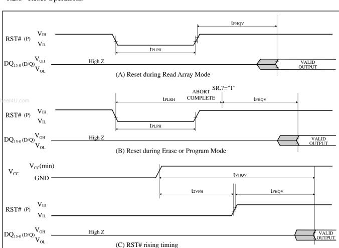
Figure 10. AC Waveform for Reset Operations
