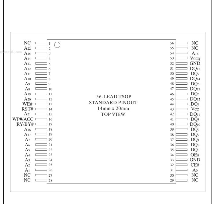
Figure 1. 56-Lead TSOP (Normal Bend) Pinout
