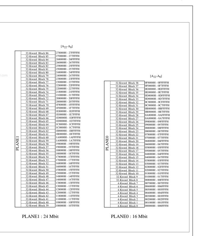
Figure 2.1. Memory Map (Bottom Parameter, Plane 0 and Plane 1)
