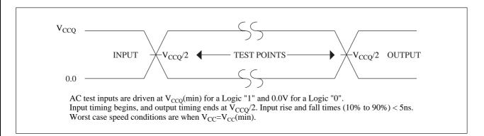
Figure 4. Transient Input/Output Reference Waveform for V<sub>CC</sub>=2.7V-3.3V
