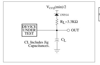
Figure 5. Transient Equivalent Testing Load Circuit
