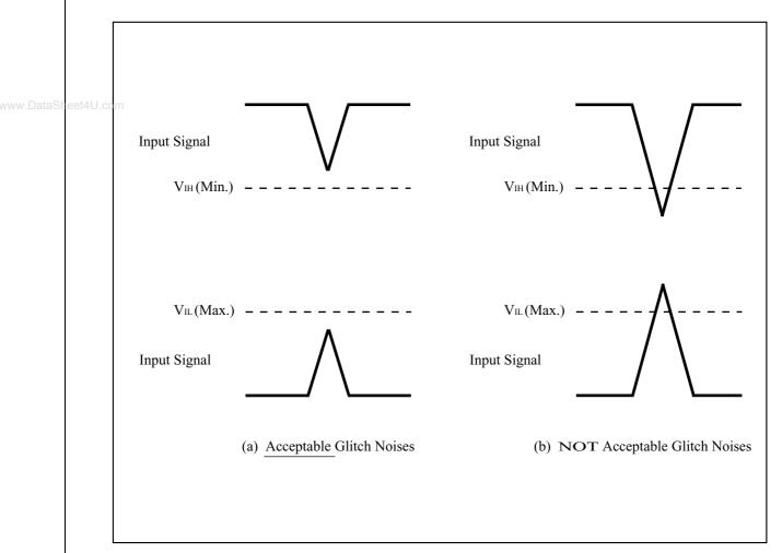
Figure A-2. Waveform for Glitch Noises
