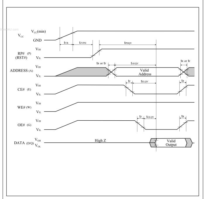
Figure A-1. AC Timing at Device Power-Up
