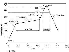
1.We recommend the reflow temperature 245°C(+/-5°C). The maximum soldering temperature should be limited to 260°C.
