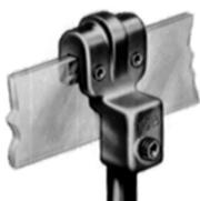
For easy installation in hard-to-reach places, these bar taps eliminate the necessity of drilling holes in the ground bus. They can be placed quickly at any location, and the only installing tool is a key wrench. A standard LOCKTITE® lug grip securely holds the tapping cable.
