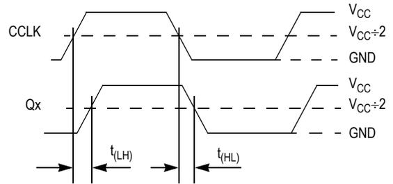
Figure 8. Propagation Delay ( $t_{PP}$ ) Test Reference
