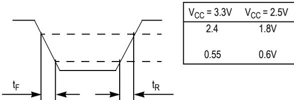
Figure 7. Output Transition Time Test Reference
