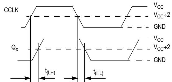
$$t_{SK(P)} = |t_{PLH} - t_{PHL}|$$
