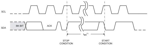
NOTE 1. The write cycle time twR is the time from a valid stop condition of a write sequence to the end of the internal clear/write cycle.
