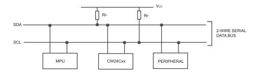
Figure 4. Typical 2-Wire Bus Configuration
