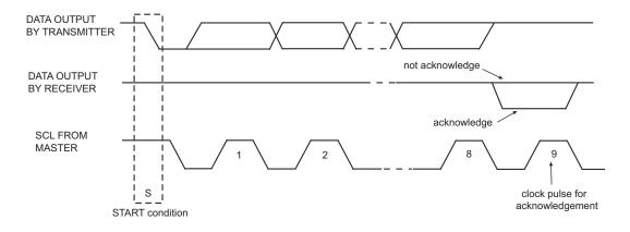
Figure 7. Acknowledge on the I<sup>2</sup>C bus
