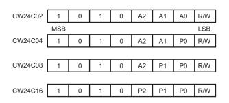
Figure 8. Device Address
