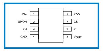
voltage will either move toward  $V_H$  or  $V_L$  depending upon the state of the UP/ $\overline{DN}$  input.
