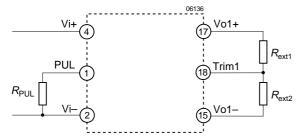
Fig. 15 Input undervoltage lockout adjustment (PUL) and output voltage adjustment by use of the Trim1 input referenced to the secondary side (triple output units).
