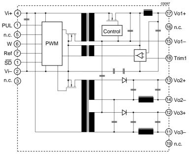
Fig. 2 Block diagram 2, triple output types
