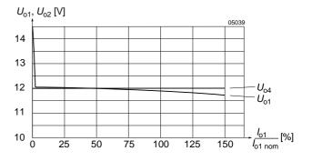
Fig. 11 Flexible load distribution on power train 1 of 40 IMX 35 D12D12-8 (4  $\times$  12 V) with load variation from 0...150% of  $P_{\text{o nom}}$  on output  $V_{\text{o1}}$  with  $V_{\text{o4}}$  loaded with 50% of  $P_{\text{o4 nom}}$ .
