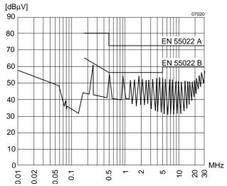
Fig. 17 Typical disturbance voltage (quasi-peak) at the input according to CISPR 11/EN 55011 and CISPR 22/EN 55022, measured at U<sub>i nom</sub> and I<sub>o nom</sub>. Output leads 0.1 m, twisted. (40 IMX 35-D12D12-9)
