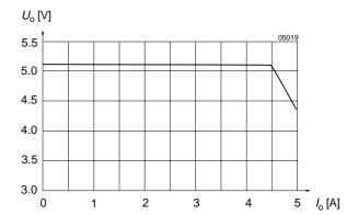
Fig. 9 a  $U_0$  versus  $I_0$  (typ) of units with  $U_0 = 5.1 \text{ V}$ . (40 IMX 35-05D12-8).
