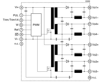
Fig. 3 Block diagram 3, quad output types
