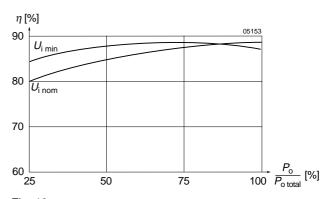
Fig. 13 Efficiency versus input voltage and load. Typical values 20 IMX 35 D12D12-8
