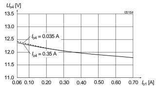
Fig. 10 Cross load regulation  $U_{04}$  versus  $I_{01}$  (typ) for various  $I_{04}$  for Vo1, Vo4 on power train 1. See: Block diagram double output types. (20 IMX 35 D12D12-8)
