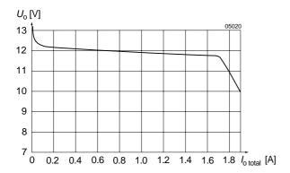
Fig. 9 b  $U_{o1/2}$  versus  $I_{o1/2}$  of double output power trains (i.e.  $2 \times 12$  V). See: Block diagram 1
