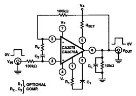
FIGURE 23. SLEW RATE, UNITY GAIN (NON-INVERTING) TEST CIRCUIT
