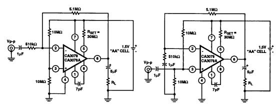
FIGURE 25. INVERTING 20dB AMPLIFIER CIRCUIT
