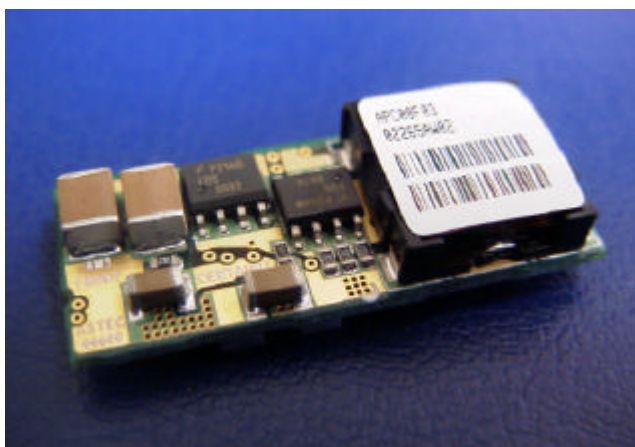
Industry Standard 0.53 X 1.3 X 0.29H SMT Package
