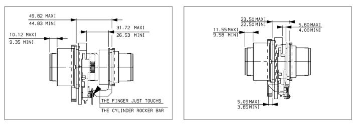
The Launching Security Device is designed to catch the floating connector plug shell during the flight.
