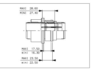
During the mating operation, the receptacle comes up to plug. The front of plug enters in receptacle cone. When plug touches the cone, this induces a lateral movement of plug shell relatively to the flange fixed on panel. This movement stops when the plug shell axis is in conformance with the receptacle ones.
