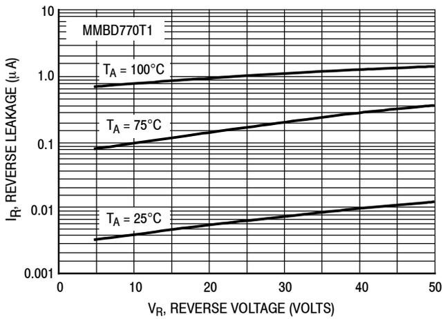
Figure 7. Reverse Leakage
