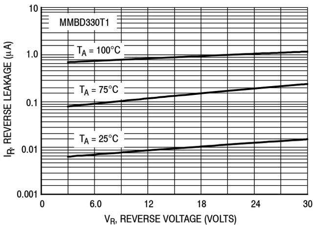
Figure 3. Reverse Leakage
