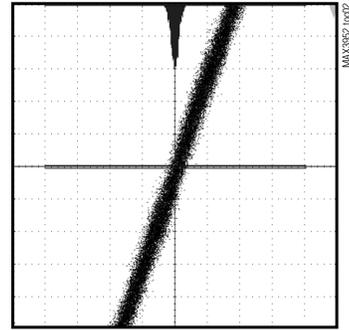
$f_{\text{REFCLK}} = 155.52\text{MHz}$ , RANDOM JITTER = 513fs<sub>RMS</sub>
