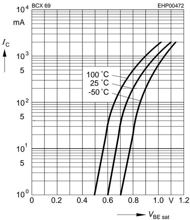
**Collector current  $I_C = f(V_{BE})$**
