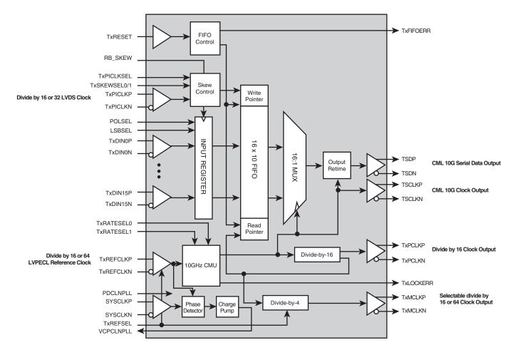
The BCM8128 is a fully integrated MSA-compliant quad-rate SONET/SDH/10GE transmitter operating at OC-192 (9.953 Gbps), 10GE (10.3125 Gbps), 10GFC (10.513 Gbps), and Forward Error Correction (FEC) data rates (10.664/10.709, 11.096, or 11.31 Gbps) with serializer and Clock Multiplication Unit (CMU). The low-jitter LVDS interface and onboard low-jitter PLL exceed Optical Internetworking Forum (OIF), IEEE 802.3ae, Telcordia, ANSI, and ITU-T jitter standards.
