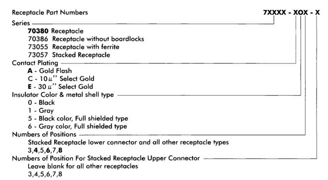
Notes: Most popular parts in bold: best availability and price. Contacts for crimp styles must be ordered separately. Plugs require pin contacts, In-line Receptacles require socket contacts. Contacts are attached to a carrier strip and supplied on reels.
