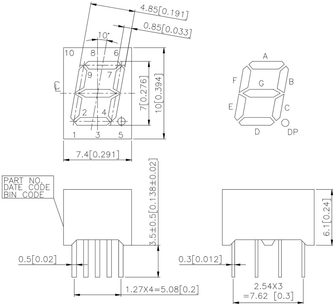
NOTES: All dimensions are in millimeters. Tolerances are ± 0.25 mm (0.01“) unless otherwise noted.
