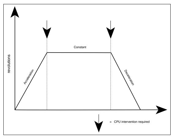
When controlling a stepper motor, providing the phase patterns onto the port pins is only part of the story. It is also necessary to modify the time between new patterns being output to allow acceleration and deceleration of the motor as shown by the velocity profile.
