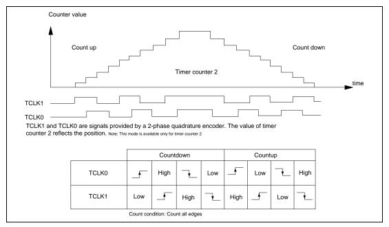
By utilising the phase counting mode on the ITU, TCNT2 will count up or down depending on the phase of the incoming signals. Therefore, the value of TCNT2 will reflect the positional changes experienced by the encoder.
