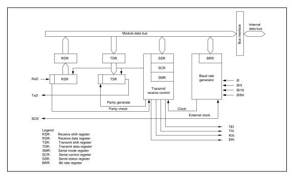
As well as using the integral Baud rate generator, each SCI can be configured to use an external serial clock.
