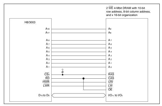
The H8/300H supports 1Mbit and 4Mbit DRAM (2WE or 2CAS) in 16-bit wide configurations. The refresh controller can be programmed to produce a wide variety of refresh intervals, and the DRAM controller can put the DRAM into self refresh mode whenever the software standby mode is selected.
