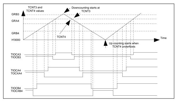
The PWM waveforms are produced from compare matches with the general registers GRB3, GRA4 and GRB4. Using this mechanism, only three registers need to be reloaded to change the modulation ratio, keeping the CPU overhead to a minimum.
