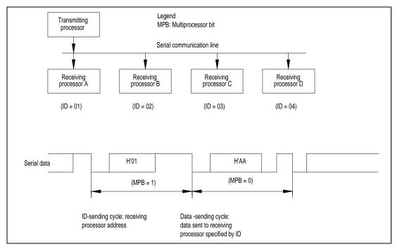
Slave devices on this network will only produce a receive interrupt when a frame is received with the MPB set, so the interrupt handler can check the address which has been transmitted.
