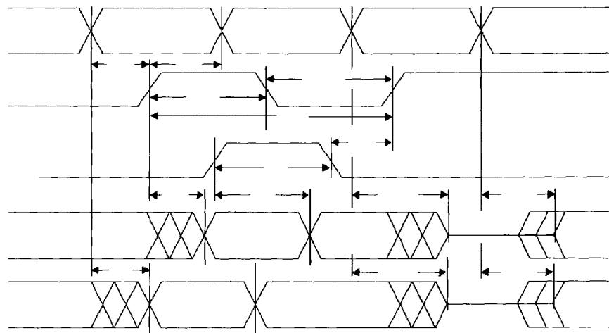
Note: 1. Timing measurement reference is 1.5 V. Input AC driving levels are 0.0 V and 3.0 V, unless otherwise specified.
