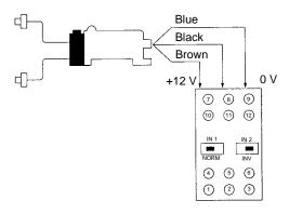
Note: A maximum of two E3X Optical Fiber Photoelectric Sensors can be connected.
