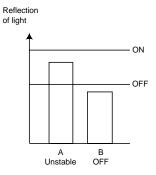
Reduce the sensitivity of the E3X with the sensitivity adjuster and turn off zone B.
