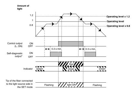
\*If the self-diagnostic output is ON when the sensing object is moving at low speed, use the E3X with an ON-delay timer circuit.
