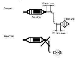
Do not apply excess force on the Fiber Units.
