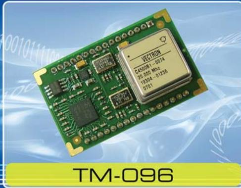
The TM-096 Integrated Timing Module is based on a digital PLL that performs filtering of the selected input signal and then synchronizes the signal to an onboard Stratum 3E OCXO. The synchronized signal is then passed through an analog PLL with an integrated VCXO in order to deliver 3 high quality output signals. Configuration and monitoring of the module's operation is achieved via an SPI interface.
