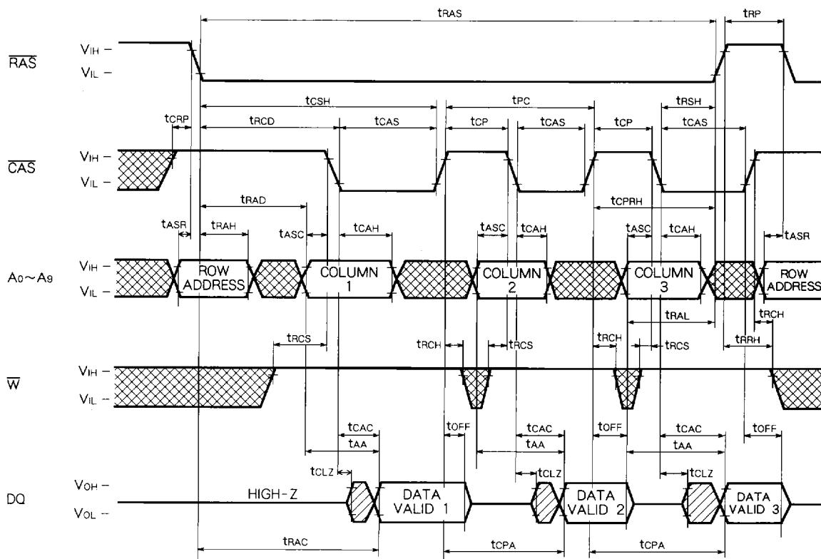
**MH1M08A0AJ-6,-7,-8/MH1M08A0AJA-6,-7,-8****FAST PAGE MODE 8388608-BIT(1048576-WORD BY 8-BIT)DYNAMIC RAM****Fast-Page-Mode Early Write Cycle**
