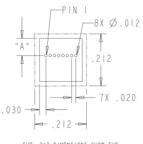
THE .212 DIMENSIONS SHOW THE MAXIMUM CERAMIC PACKAGE ENVELOPE (INCLUDING ALIGNMENT TOLERANCES) RELATIVE TO OSA.
