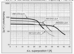
dc-current pre-loadability <Example> •Core : W462725J2, Frequency : 100 kHz
