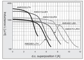
dc-current pre-loadability (3) <Example> •Core : C462720J2, C462725J2, Frequency : 100 kHz
