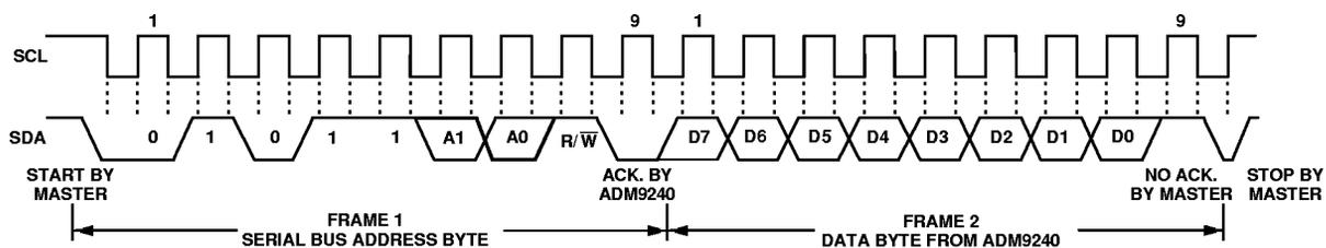
Figure 2c. Reading Data from a Previously Selected Register
