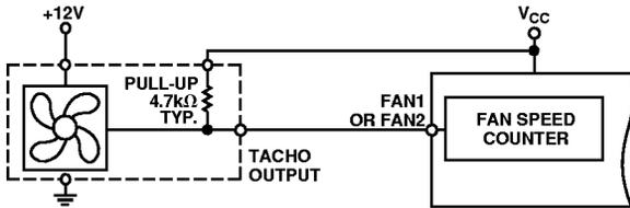
Figure 6a. Fan with Tachometer Pull-Up to  $+V_{CC}$
