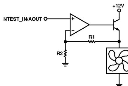
Figure 5. Analog Output Driving Fan
