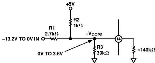
Figure 4. Scaling  $V_{CCP2}$  to  $-12\text{ V}$  ( $\pm 10\%$ )
