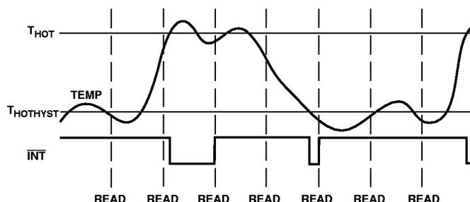
Figure 11.  $\overline{\text{INT}}$  Output in One-Time Interrupt Mode
