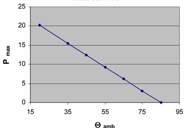
Max. allowable current (rms) at specific ambient Temp.
