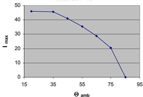
Max. allowable ambient Temp. at specific power loss
