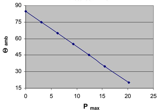
Max. allowable ambient Temp. at specific current (rms)
