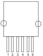
Pin 1: External Offset Adjust Pin 2: VS Pin 3: + Output Pin 4: Ground Pin 5: N/C Pin 6: N/C
