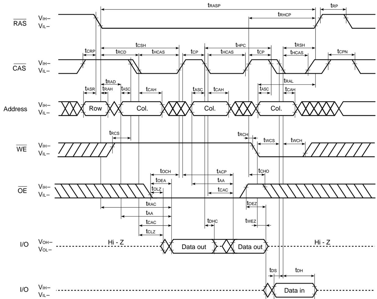
**Remark** In the hyper page mode (EDO), read, write and read modify write cycles are available for each of the consecutive  $\overline{\text{CAS}}$  cycles within the same  $\overline{\text{RAS}}$  cycle.
