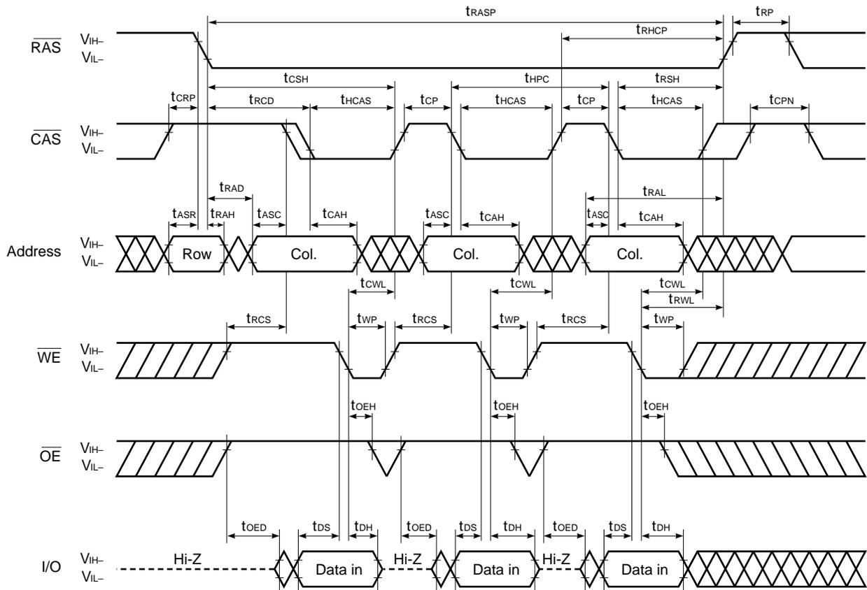
**Remark** In the hyper page mode (EDO), read, write and read modify write cycles are available for each of the consecutive  $\overline{\text{CAS}}$  cycles within the same  $\overline{\text{RAS}}$  cycle.
