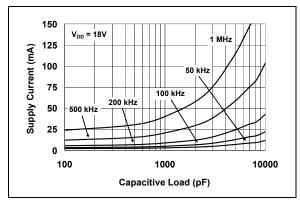
FIGURE 2-13: Supply Current vs. Capacitive Load.
