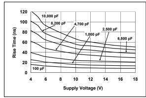
**FIGURE 2-1:** Rise Time vs. Supply Voltage.
