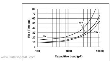
FIGURE 2-2: Rise Time vs. Capacitive Load.
