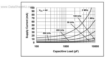
FIGURE 2-15: Supply Current vs. Capacitive Load.
