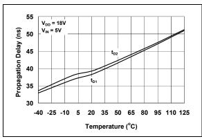
**FIGURE 2-8:** Propagation Delay Time vs. Temperature.
