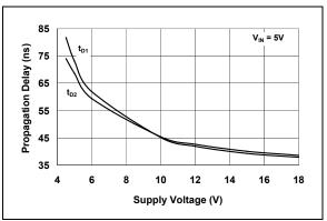
**FIGURE 2-6:** Propagation Delay vs. Supply Voltage.
