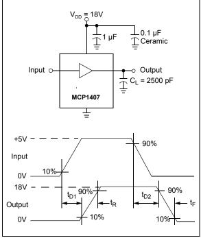
**FIGURE 4-2:** Non-Inverting Driver Timing Waveform.
