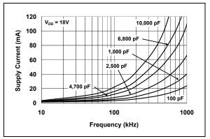
**FIGURE 2-16:** Supply Current vs. Frequency.
