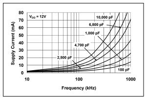
FIGURE 2-17: Supply Current vs. Frequency.
