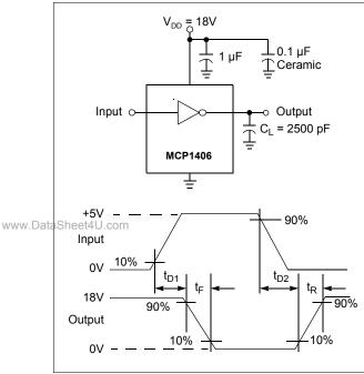
**FIGURE 4-1:** Inverting Driver Timing Waveform.
