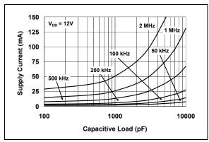
FIGURE 2-14: Supply Current vs. Capacitive Load.
