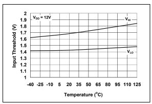
**FIGURE 2-12:** Input Threshold vs. Temperature.
