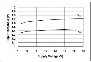
FIGURE 2-11: Input Threshold vs. Supply Voltage.
