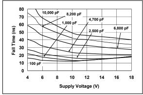
**FIGURE 2-4:** Fall Time vs. Supply Voltage.
