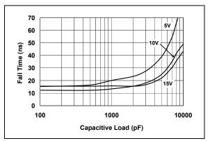
**FIGURE 2-5:** Fall Time vs. Capacitive Load.
