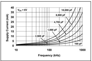
FIGURE 2-18: Supply Current vs. Frequency.
