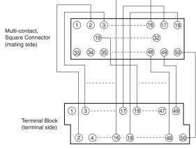
Note: All pins on the Multi-pole, Square Connector correspond 1-to-1 to the terminal of the same number on the terminal block as shown above.
