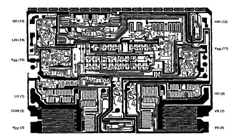
Die bonding pad locations and electrical functions
