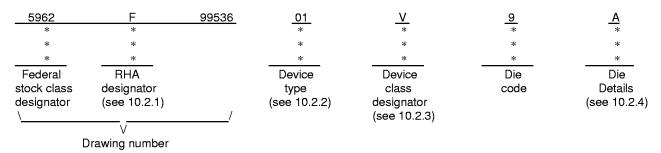
10.2.1 <u>RHA designator</u>. Device classes Q and V RHA identified die shall meet the MIL-PRF-38535 specified RHA levels. A dash (-) indicates a non-RHA die.
