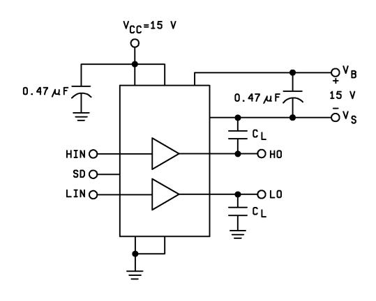
FIGURE 4. Switching time test circuit.
