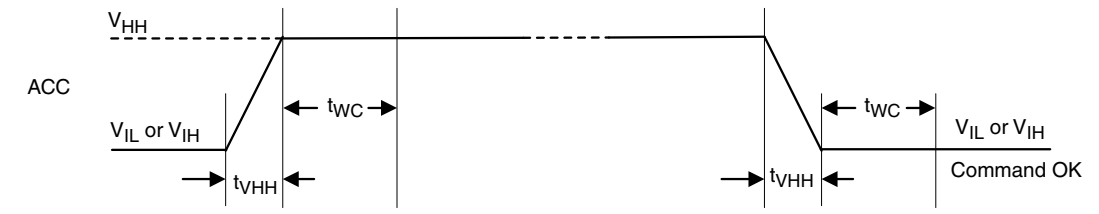
Figure 13.1 ACC Program Acceleration Timing Requirements
