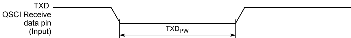
Figure 10-13 TXD Pulse Width
