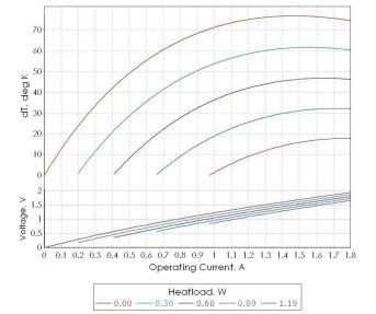
**Note**: Performance data is specified at optimal optimal conditions (TEC hot side is stabilized at ambient temperature). Any heatsink thermal resistance is not included into estimations. Use TECCad Software for estimations under different conditions.
