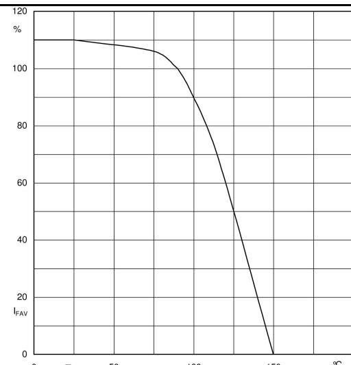
Fig. 2 Rated forward current vs. temp. of the terminals<sup>4)</sup>
