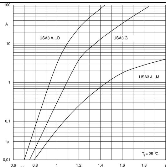
Fig. 1 Forward characteristics (typical values)
