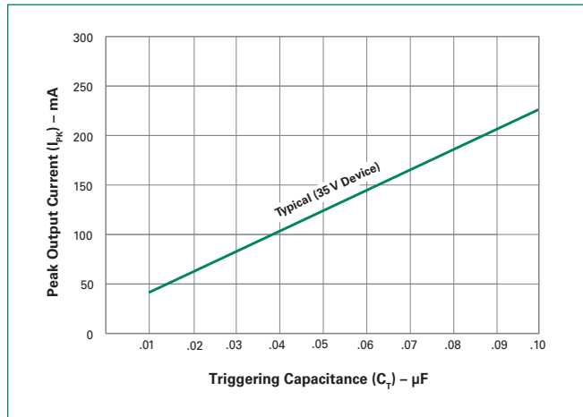
Figure 7: Peak Output Current vs. Triggering Capacitance (Per Figure 5 with R_L of 20 Ω)
