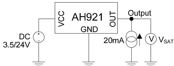
Figure 9. Test Condition of AH921 (Output Saturation Voltage)
