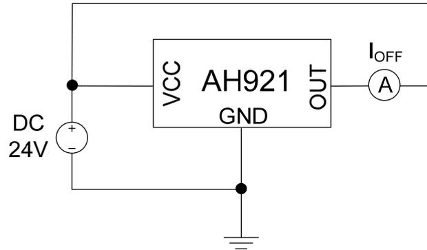
Figure 10. Test Condition of AH921 (Output Leakage Current)
