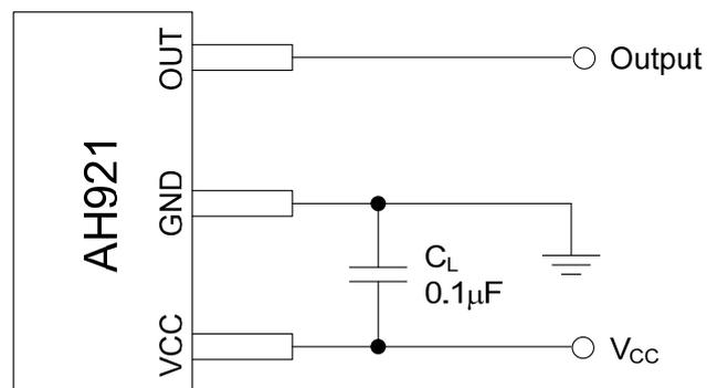
Figure 7. Test Circuit of AH921
