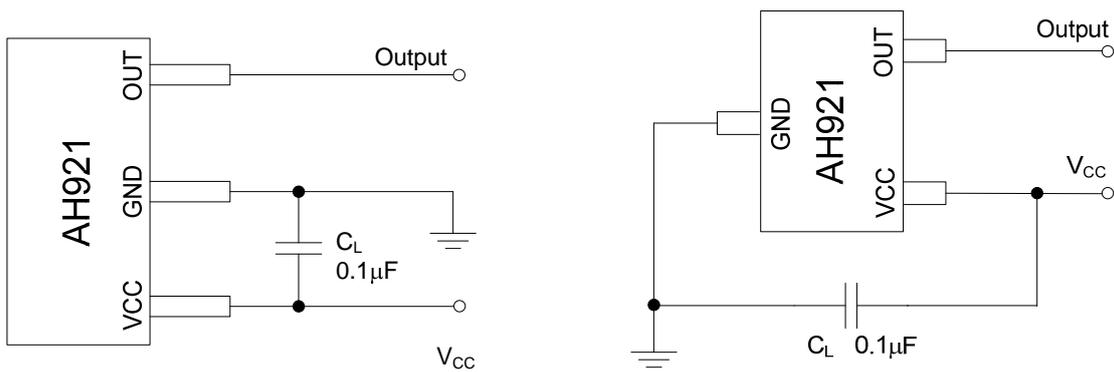
Figure 18. Typical Application Circuit of AH921
