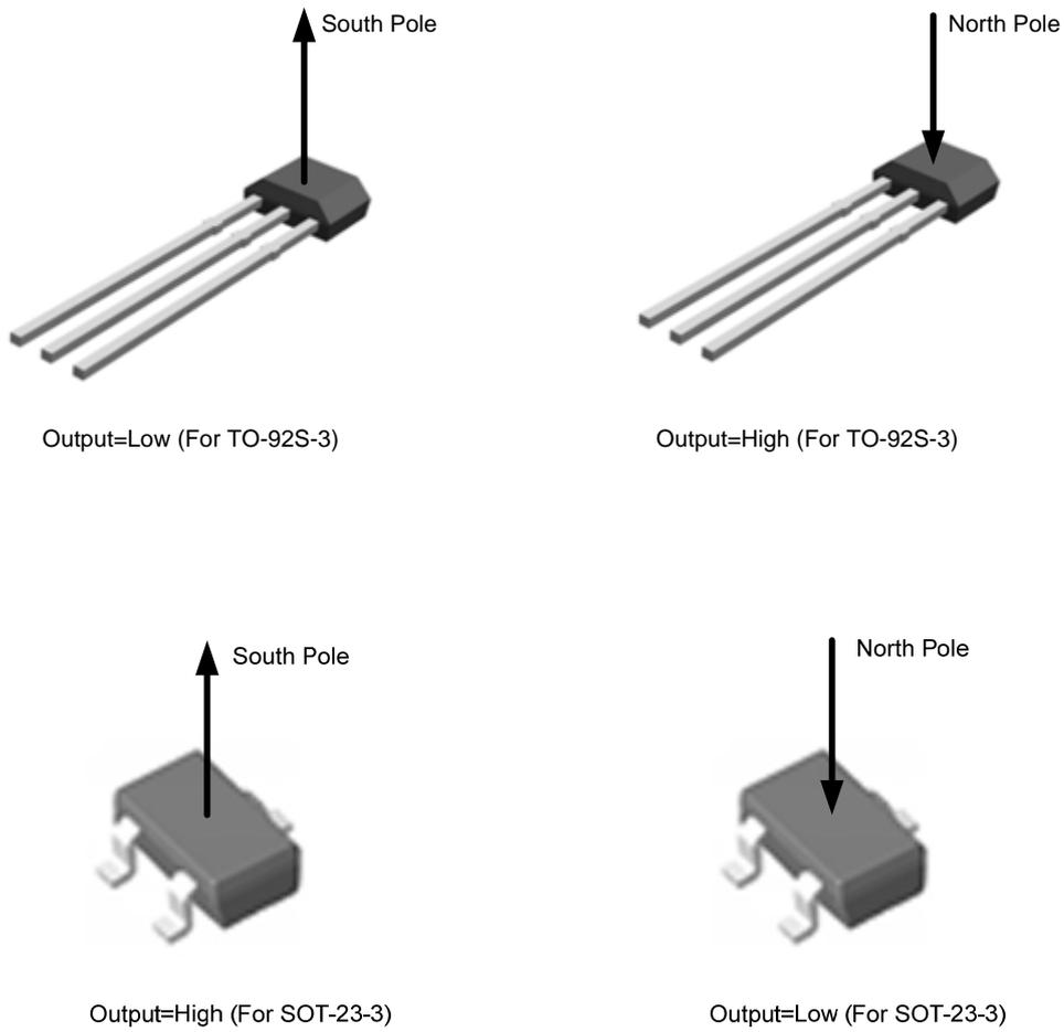
Figure 5. Output Status vs. Magnetic Pole
