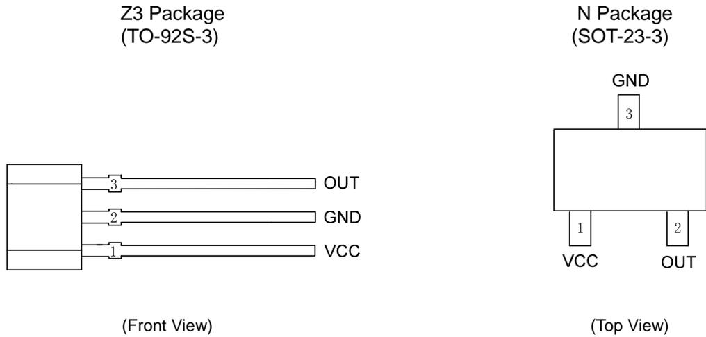
Figure 2. Pin Configuration of AH921
