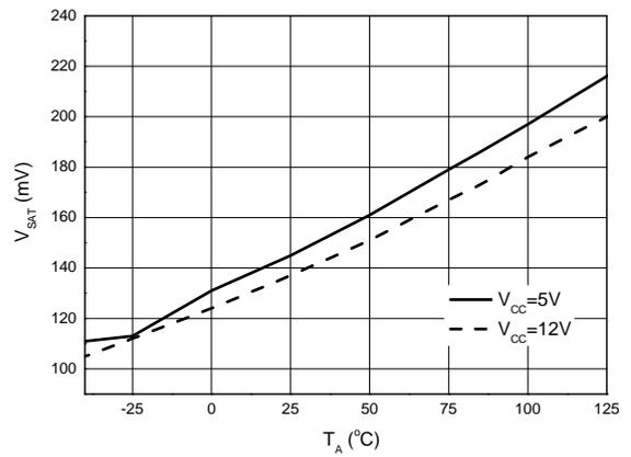
Figure 16. V<sub>SAT</sub> vs. T<sub>A</sub>
