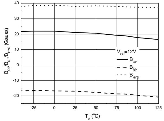
Figure 14. B<sub>OP</sub>/B<sub>RP</sub>/B<sub>HYS</sub> vs. T<sub>A</sub>
