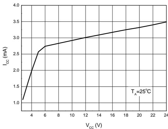
Figure 11. I<sub>CC</sub> vs. V<sub>CC</sub>
