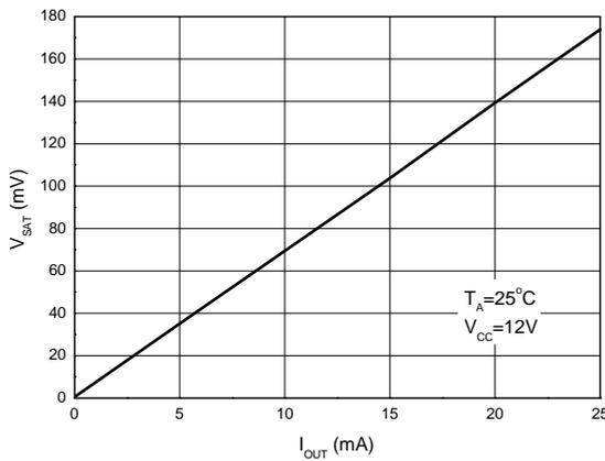
Figure 15. V<sub>SAT</sub> vs. I<sub>OUT</sub>
