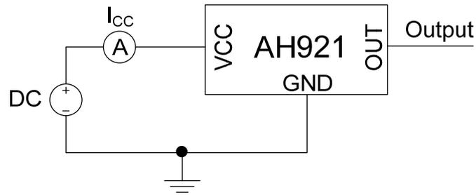
Figure 8. Test Condition of AH921 (Supply Current)
