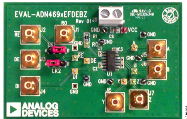
Figure 15. EVAL-ADN469xEFDEBZ Customer Evaluation Board
