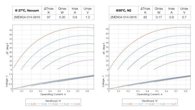
**Note**: Performance data is specified at optimal conditions (TEC hot side is stabilized at ambient temperature). Heatsink thermal resistance is not included into estimations. Use TECCad Software for estimations under different conditions.
