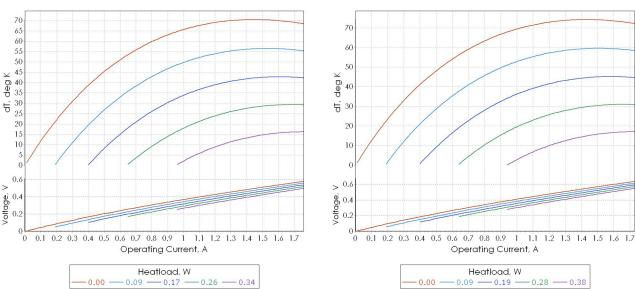
**Note**: Performance data is specified at optimal optimal conditions (TEC hot side is stabilized at ambient temperature). Any heatsink thermal resistance is not included into estimations. Use TECCad Software for estimations under different conditions.
