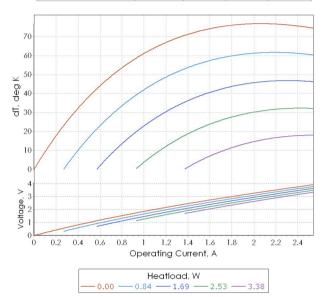
**Note**: Performance data is specified for optimal optimal conditions (TEC hot side is stabilized at ambient temperature). Heatsink thermal resistance is not included into estimations. Use TECCad Software for estimations under different conditions.
