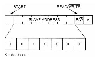
Figure 5. Control Byte Allocation
