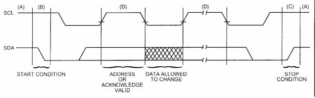
Figure 4. Data Transfer Sequence on the serial bus
