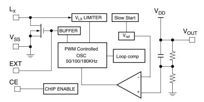
$V_{\it DD}$  is internally connected to the  $V_{\it OUT}$  pin.
