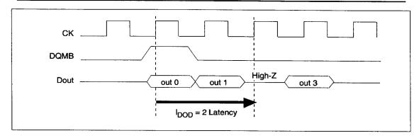
Writing: Input data can be masked by DQMB. By setting DQMB to Low, data can be written. In addition, when DQMB is set to High, the corresponding data is not written, and the previous data is held. The latency of DQMB during writing is 0.
