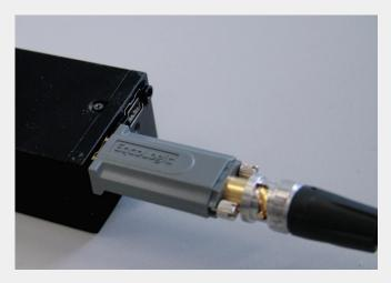
When using the dongles, customers can determine the best cable lengths for their applications. The EqcoLogic transceiver contains an equalizer that is fully adaptive and adjusts for various cable lengths as well as age and environmental conditions like temperature, without any need for programming. The dongles have a standard 1394b 9-pin connector on one end and a  $75\Omega$  BNC or  $50\Omega$  SMA connector on the opposite end.
