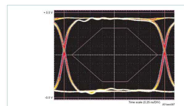
Fig 10. Eye-pattern 480 Mbps USB signal with no switch.
