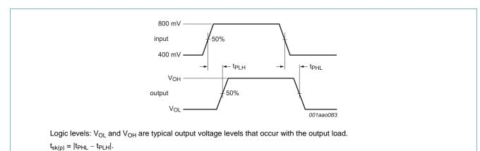
Fig 6. The data input to output propagation delay times and pulse skew time
