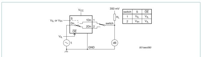
Adjust f<sub>i</sub> voltage to obtain 0 dBm level at output. Increase f<sub>i</sub> frequency until dB meter reads -3 dB.
