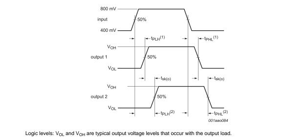
Logic levels. Vol. and VoH are typical output voltage levels that occur with the output load
